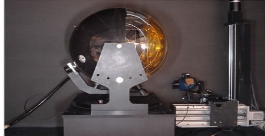
inside: OM, light source, motor
