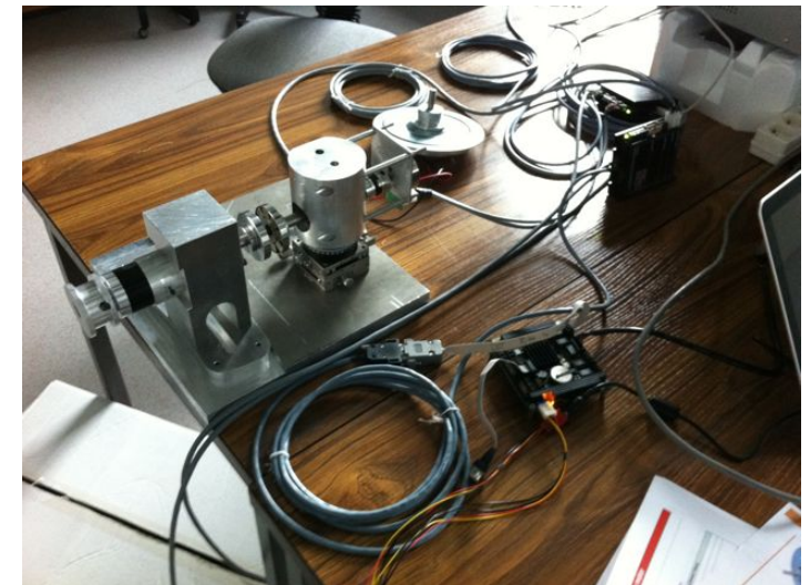
Spring 2012 : Control of the motor / magnetic transmission of the carousel-filter un-clamp system 20
